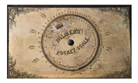
The first calculating rule of American design. A most unusual and ingenious calculating device published by Aaron Palmer who is best known for his large circular nomograph calculating boards. This pocket calculator, however, is based on two logarithmic scales laid out in a circular pattern. The scales rotate against one another and are affixed to a heavy card stock and mounted to the
